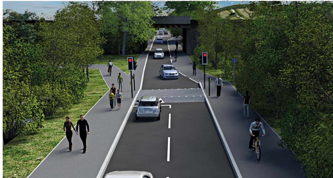
Visualisation of possible shared use footway/cycleway under the rail bridge on The Straight Mile, looking towards Hereford Enterprise Zone. Shows toucan crossing and the priority working for motor vehicles under rail bridge
