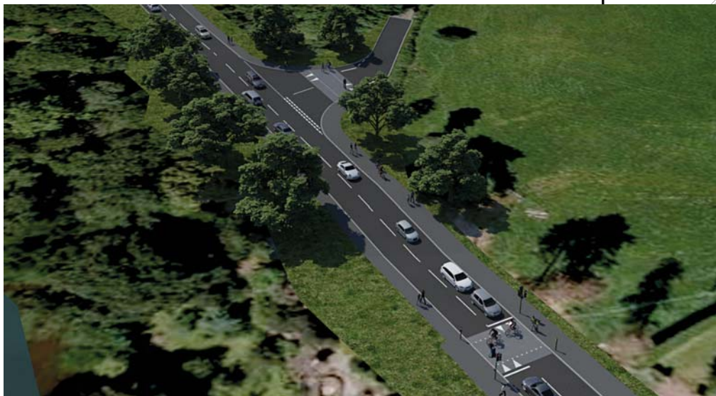
Visualisation looking northwest of possible walking and cycling improvements at western end of Belmont Road. Shows possible Toucan crossing of Belmont Road and improvements at junction with Ruckhall Lane
